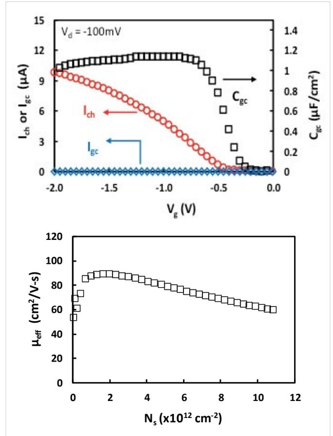
Figure 6. (a)  $I_{ch}$ ,  $I_g$ , and  $C_{gc}$  extracted simultaneously from the currents in Figure 5 by using Equations (2)–(5). (b) Channel effective mobility extracted from  $I_{ch}$  and  $C_{gc}$  from (a).
