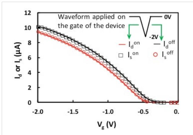
Figure 5. Four currents measured from source and drain corresponding to the off-to-on and on-to-off  $V_g$  sweep. Schematic  $V_g$  waveform is shown in inset.
