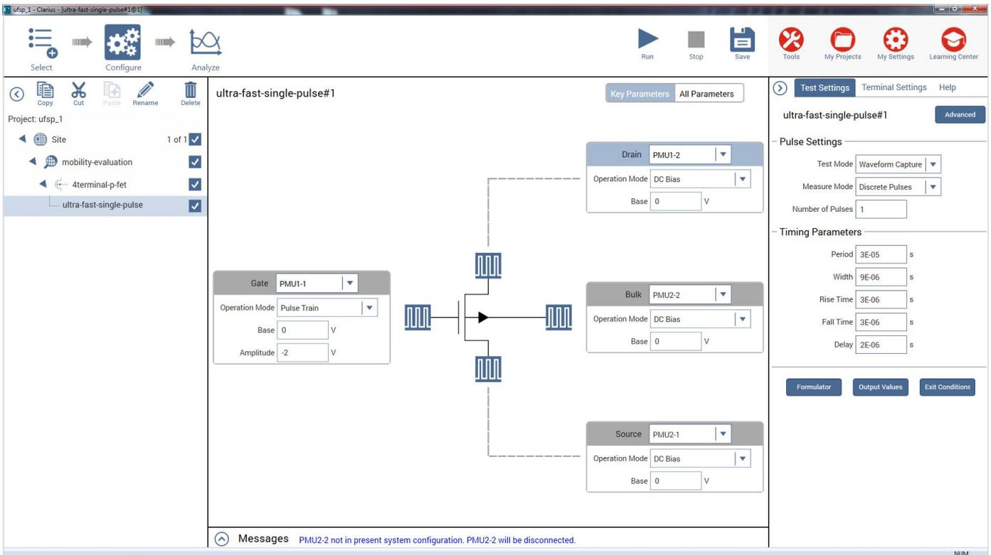
Figure 12. Example project in the Clarius software for UFSP measurement. Each of the four terminals of the device is connected to one channel of PMU respectively.
